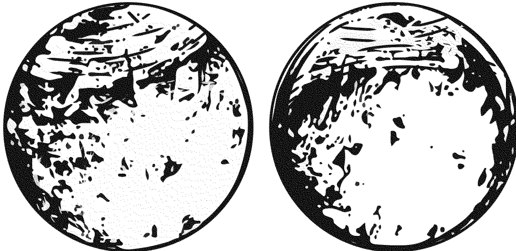
Figure D-4. Fatigue failure, no stress, and high stress concentration
